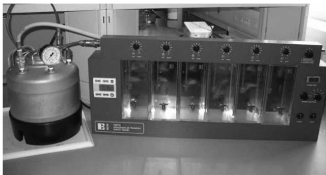
Figure 2. Photograph of the bench scale dissolved air flotation jar tester (EC Engineering Dissolved Air Flotation Batch Tester, Model DBT6).
